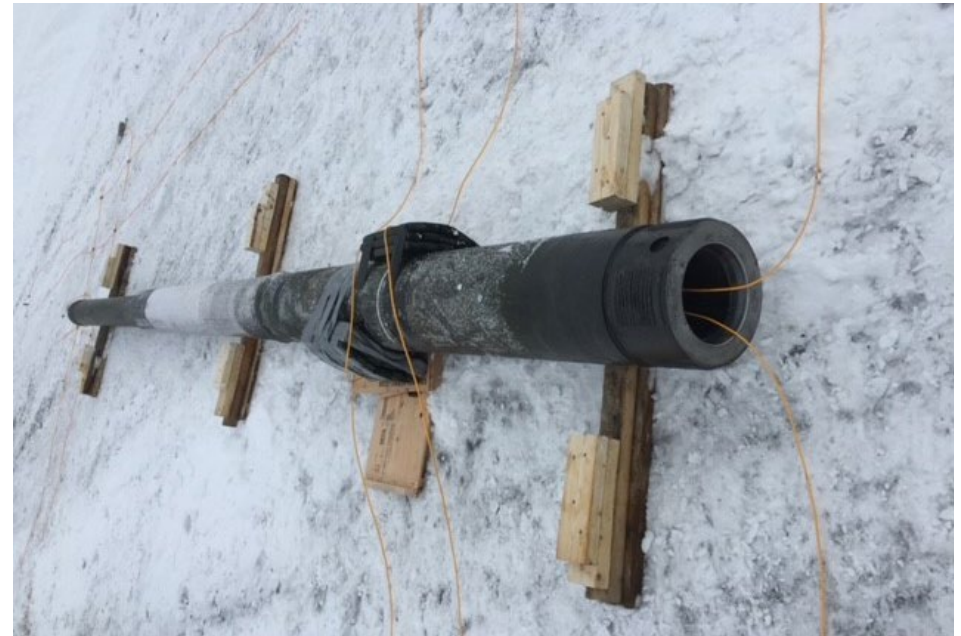
Note the M777 barrel loaded with explosives above and a large piece of barrel post-detonation below.
